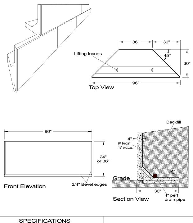
Concrete Min. Strength: 4,000 psi at 28 days Reinforcement: #4 Rebar Air Entrainment: 6% Weight: 2' = 1,500 lbs, 3' = 1,900 lbs 1/2 Section can be made with left half only
